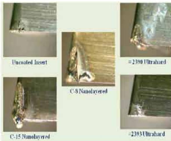
(C) FEED RATE - 0.100 MM/REV
