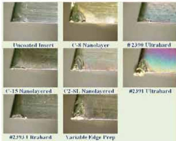
(B) FEED RATE - 0.075 MM/REV
