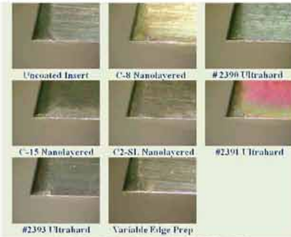
(A) FEED RATE - 0.050 MM/REV
