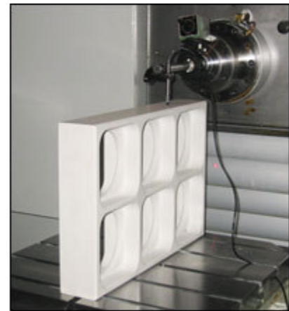
Master ceramic square for pitch error is shown. Angular and straightness errors can be detected by use of a ceramic square, electronic levels, and laser interferometers.
